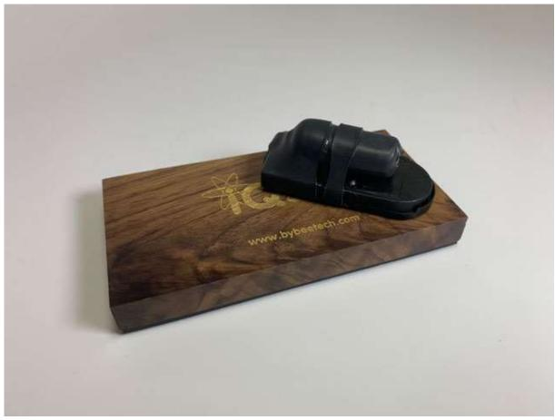
The Version 2 is odd looking, resembling an oversized beetle, about 2" long, 1" wide and 1" tall. It is built on a flat plastic surface which is also a battery pack. The device consumes so little energy that the pack should last a lifetime.
